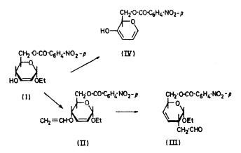
and the ethanol generated was continually removed by codistillation with pentane. A crystalline product was obtained in 30% yield (after chromatography) which had an n.m.r. spectrum indicative of the monovinyl ether structure (II). Heating this ether in nitrobenzene at 185° for 3.5 h caused its complete conversion into a chromatographically distinguishable product which, after isolation, was shown to have reducing
